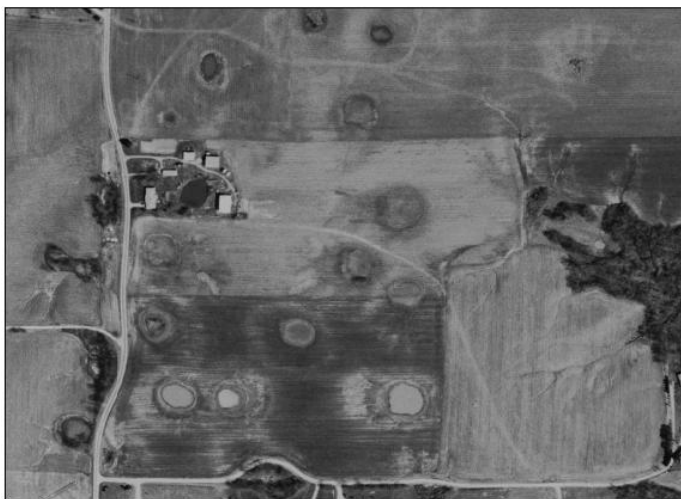
Figure 2. Numerous sinkholes and sinkhole ponds are seen in this aerial photo of a farmstead in the karst sinkhole plain of southwestern Illinois.
